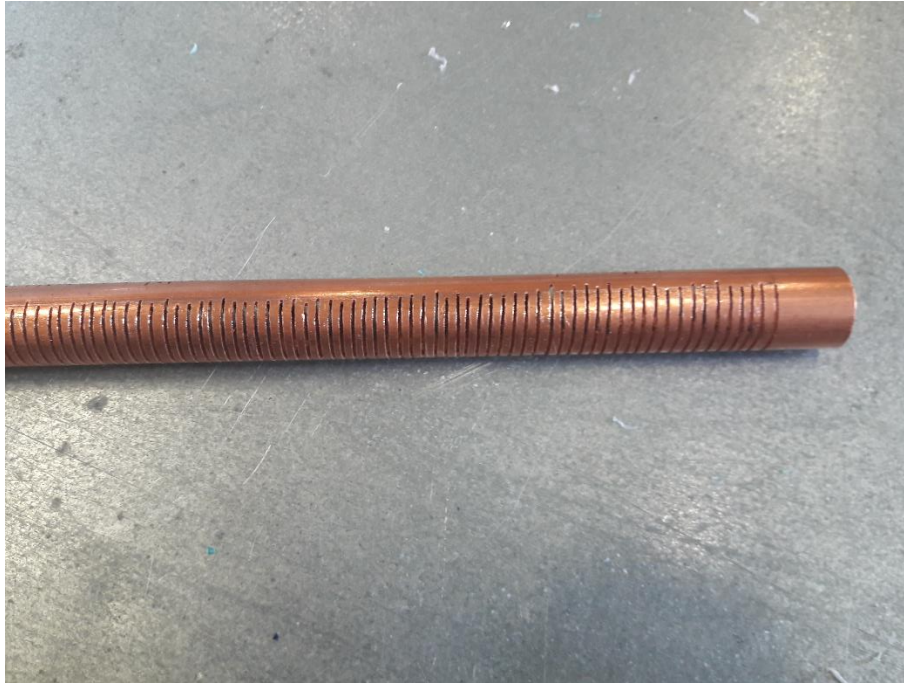
Figure 3.6. Photograph of copper pipe gas injector design.
