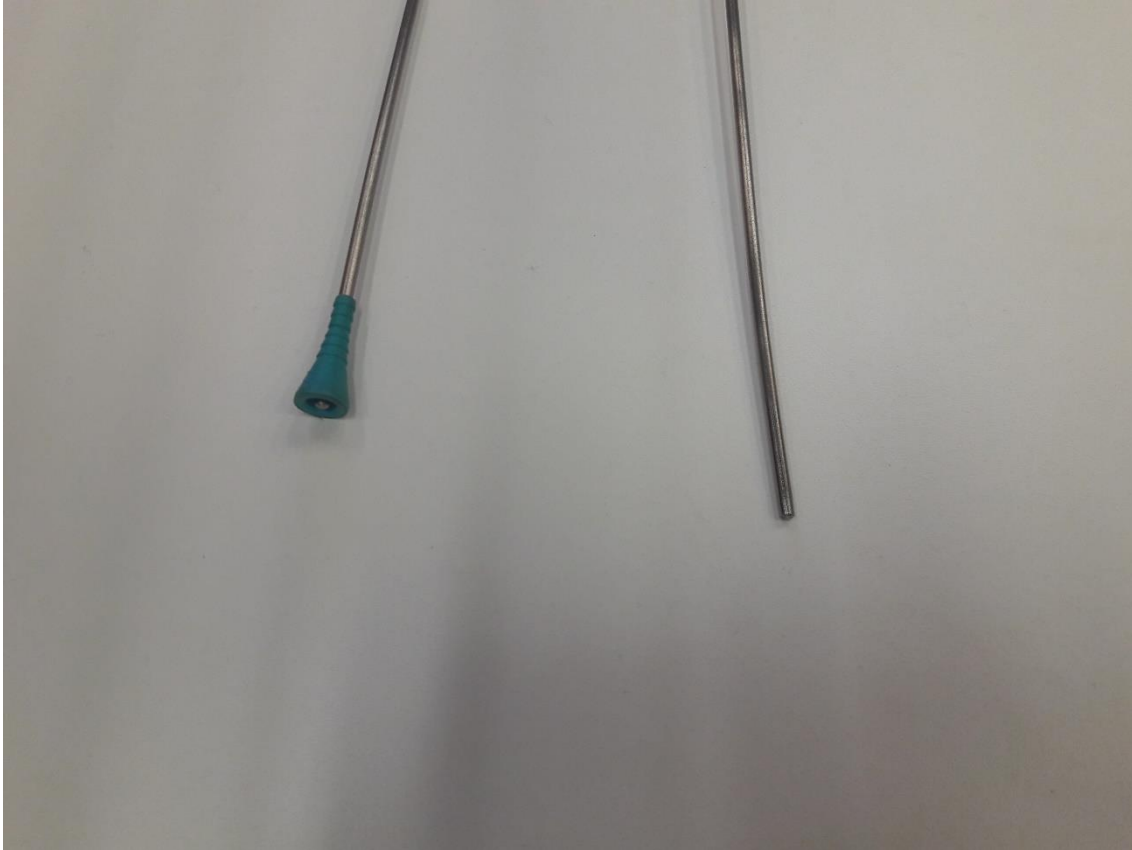
Figure 3.3. Image of thermocouple with shroud.
