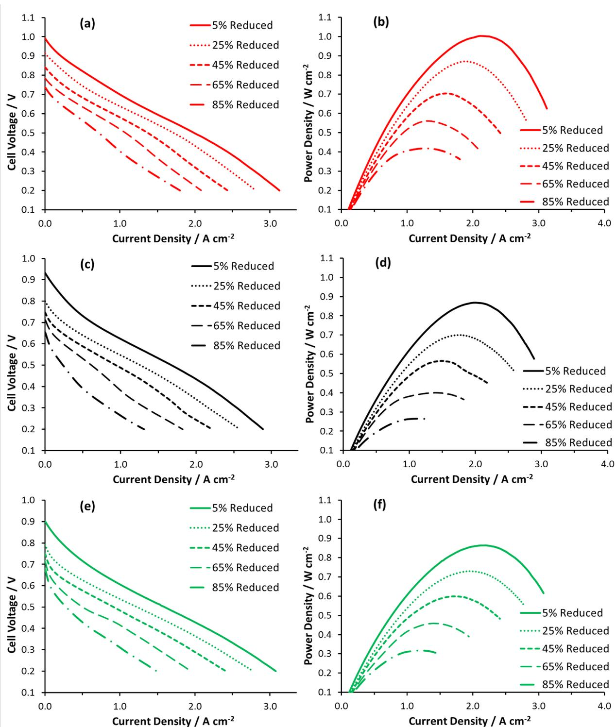
**Figure S3.** (a) *i*-*V* and (b) corresponding power density curves generated with 0.3 M HV3 at varying levels of reduction. (c) *i*-*V* and (d) corresponding power density curves generated with 0.3 M NaV3 at varying levels of reduction. (e) *i*-*V* and (f) corresponding power density curves generated with 0.3 M NaV4 at varying levels of reduction.
