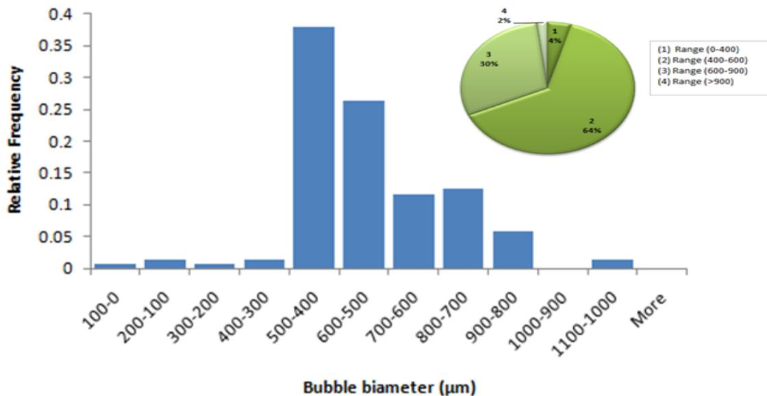
Figure 2: Bubble size distribution using the ceramic diffuser for the air/water system at 300 ml/min
