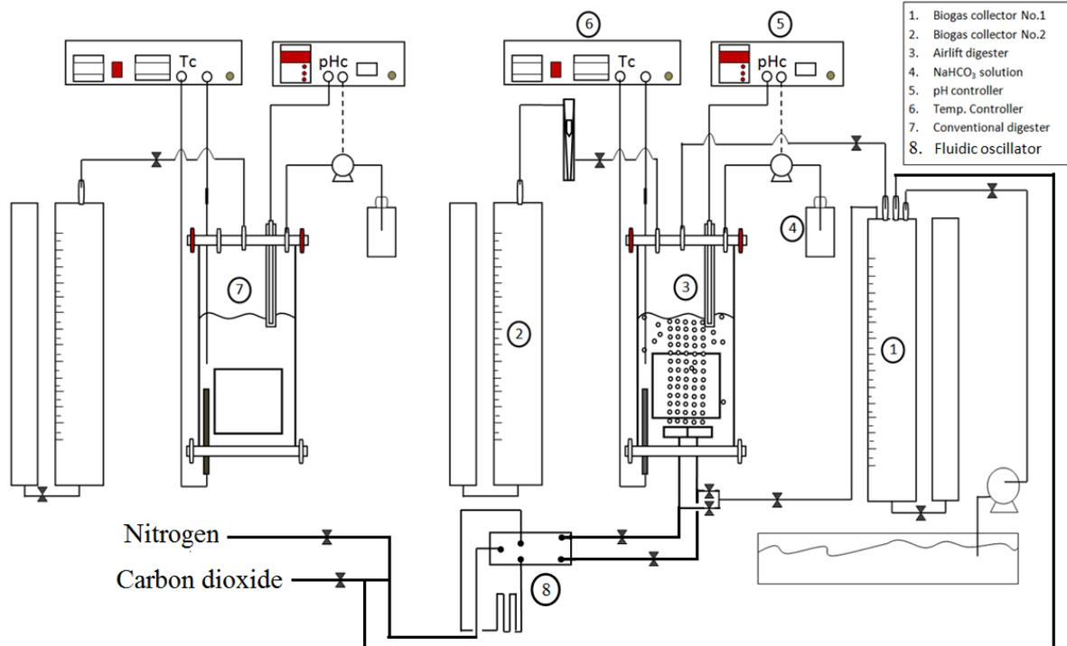
Figure 1: Schematic of experimental work. Two digesters: a gaslift (or airlift) digester and an unsparged digester as a control are compared in this work. Sparging is carried out using carbon dioxide rich microbubbles, with composition a controlled variable with five different levels from 0-100% CO<sub>2</sub>.
